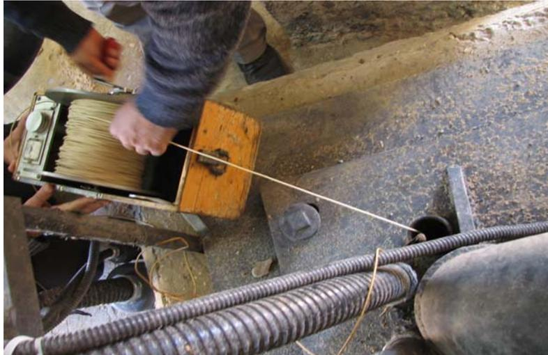
**Figure 6.5** Measuring water level by M-scope
