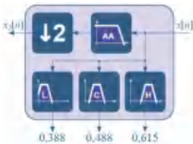
Figure 6. Base block used to build the bank filter. Frequencies are normalized to sampling frequency ( F_s/2 ).
