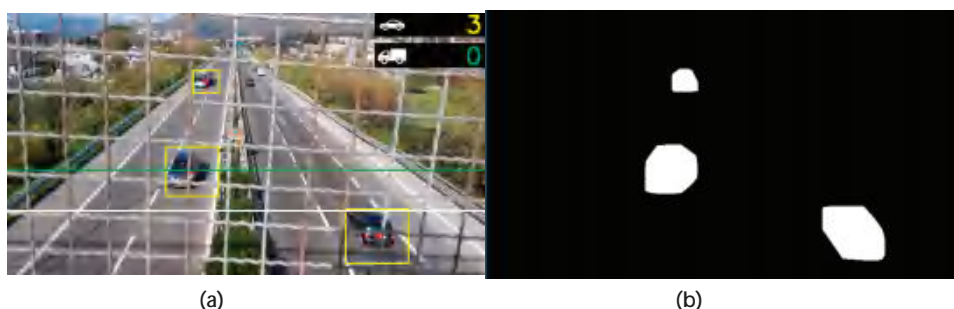
Figure 1. Image analysis on the video frame. (a) Moving object are bounded in a yellow box and a red dot (centroid) is applied. Green and white line are used for counting and speed estimation; (b) blob detection after background subtraction.
