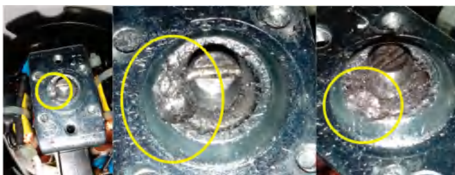
Figure 8. CG-A with a heavily damaged rear sliding bearing (indicated by yellow circle).
