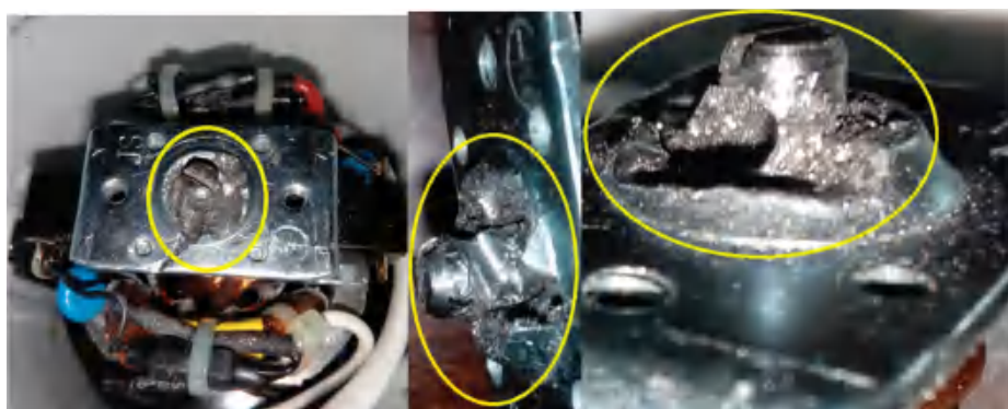
Figure 9. CG-A with a damaged shaft and heavily damaged rear sliding bearing (indicated by yellow circle).
