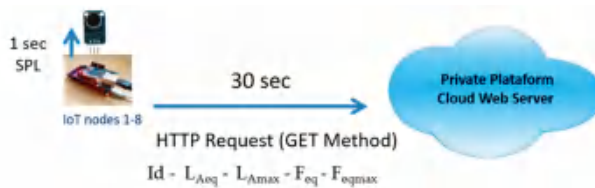
Figure 8. The Hyper Text Transfer Protocol (HTTP) request—GET method.
