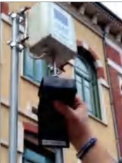
Figure 10. Operation of calibration on DYNAMAP sensor.
