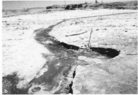
Fig. 5.2. a Childress County, Texas, Jonah Creek, a tributary of Red River. Spring discharge prior to initiation of pumping test. b Cessation of discharge from spring during pumping test
