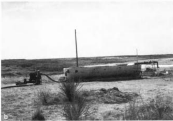
Fig. 5.1. a Childress County, Texas, Jonah Creek, a tributary of Red River. Instrumentation for measurement of water levels and monitoring discharge during pumping test. b Pumping test in progress
